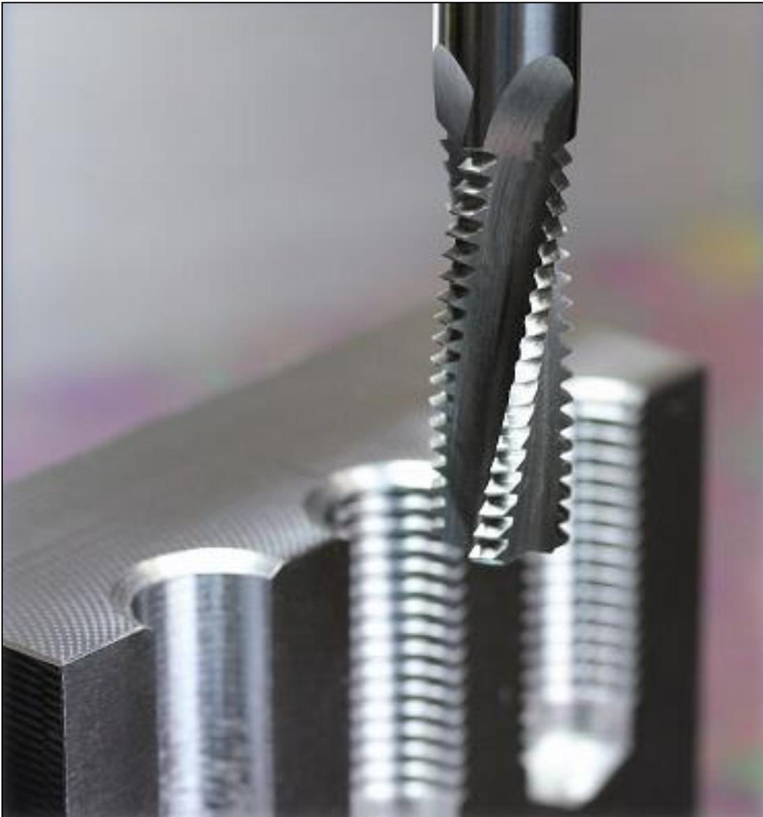
*Figura 36.* Fresado de roscas. Fuente: <http://www.hydratight.com/es-mx/resources/news/2009/01/hydratight-s-industry-leading-portable-thread-milling-service-now-us>
